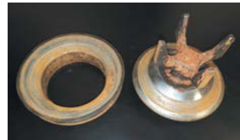
/ Typical valve and upper seat with more than 80 hours @ 10,000 psi and 100 mesh
